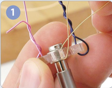
1 Place up to 5 Artistic Wires onto the disc of the Wire Twister, then attach the wires to a sturdy object.
