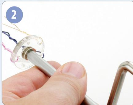
2 Pull the wires taut, turn the crank, and watch the wires twist.
